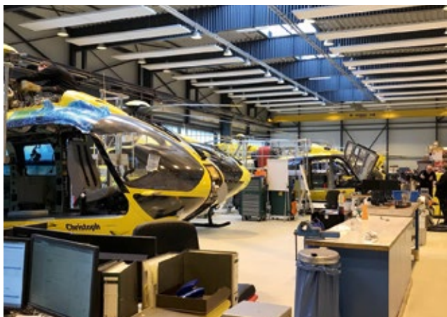
Helicopters are everywhere at ALT: these machines are waiting for inspection in ten different bays.
